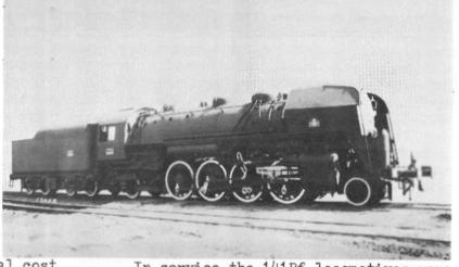
In service the 141Rf locomotives were capable of pulling 600-ton passenger jobs at 65 miles-per-hour or 1500-ton freights at 30 mph. The design of this class incorporated a perfect combination of simplicity and modernity. As recently as 1969 hundreds of these 2-8-2's were still storming the French countryside, although few remain today.
